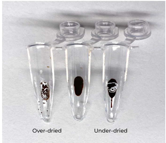
Figure 2. Over-dried beads are cracked and flakey, resembling dried mud. Under-dried beads are glossy and wet, like saturated mud. Optimally dried beads appear damp, but lack gloss.
