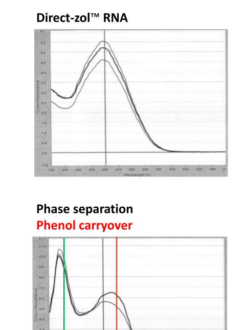
No phenol carryover with Direct-zol™ RNA. RNA isolated by conventional phase separation method shows phenol contamination as indicated by the absorption peak at 230nm (green) and peak shift 260->270nm (red).
