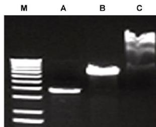
Ultra-pure DNA from the **DNA Clean & Concentrator** can be easily ligated for efficient cloning. Lanes: A: 3.5 kb blunt-ended vector; B: 7.4 kb blunt-ended DNA insert; C: Blunt-end ligation of A+B mixture.
