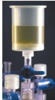
**Vacuum:** Zymo-Spin VI<sup>™</sup> Column connected to a vacuum manifold.
