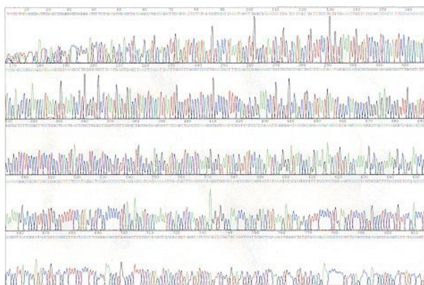
Sequencing chromatogram of pGEM® DNA generated using an ABI 3730xl DNA analyzer. DNA was labeled with ABI BigDye Terminator v3.1 and cleaned using the ZR DNA Sequencing Clean-up Kit™ .
