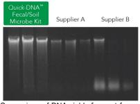
Comparison of DNA yields from rat feces using the *Quick*-DNA™ Fecal/Soil Microbe Kit and kits from suppliers A and B. Equivalent amounts of feces were processed using each kit and then equal volumes of eluted DNA were analyzed in a 0.8% (w/v) agarose/ethidium bromide gel. Samples were processed in triplicate.
