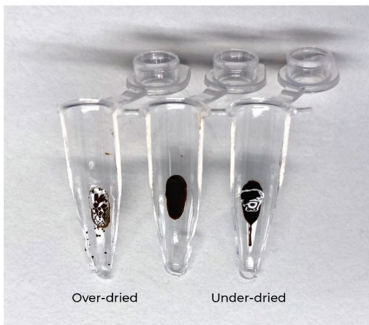
Figure 5. Examples of over-dried, optimally dried, and under-dried Select-a-Size MagBeads. Over-dried beads are cracked and flakey, resembling dried mud. Under-dried beads are glossy and wet, like saturated mud. Optimally dried beads appear damp, but lack gloss.
